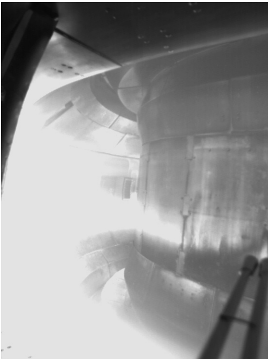
Fig. 1. He-ICR plasma in presence of 1 Tesla of toroidal magnetic field in EAST (CCD picture).
